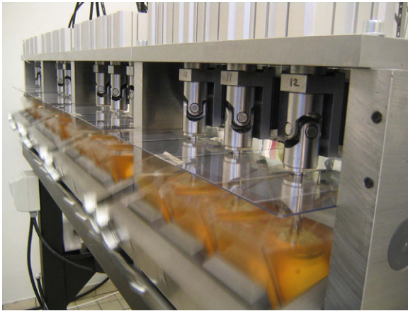
Fig. 1. HUT-4 anatomic hip joint simulator running with 12 stations and the test chambers filled with 500 ml of serum-based lubricant in each. The universal joints making acetabular inserts self-centering on femoral heads are clearly visible above the test chambers. On the top of the simulator are the pneumatic loading cylinders.
