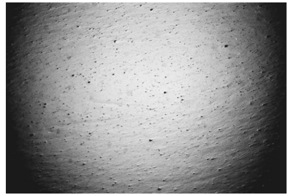
Fig. 8. Optical micrograph from contact zone of femoral head of Stafit 60° test after 5 mc. There are no wear marks. Picture width corresponds to 2 mm.
